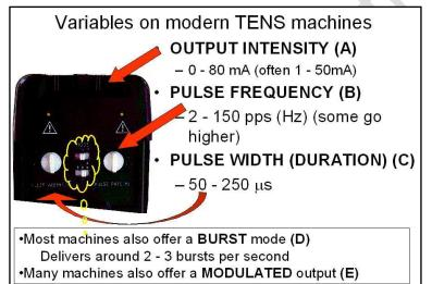
variables which are available on modern machines will be outlined. The location of these controls on a typical (analogue) TENS machine is illustrated in the diagram below.
